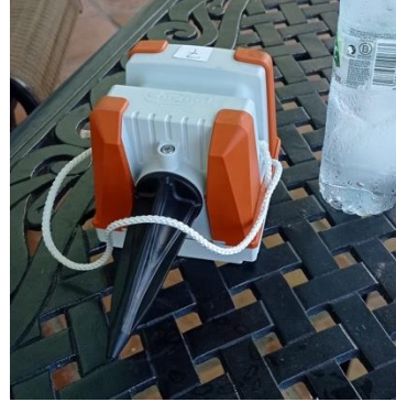
120 autonomous seismic nodes (£0.3k) (Sercel, WiNG, DFUs)
